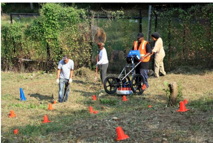
Pierce Park Archaeology team at work with ground penetrating radar
